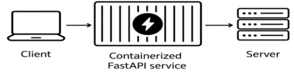
Figure 3: Deployment architecture of the phishing detection system. A client sends a text query to the containerized FastAPI service, which hosts the fine-tuned model and returns the predicted label and confidence score to downstream servers.
